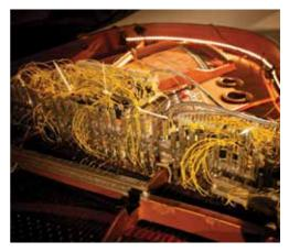
together with the Magnetic Resonator Piano (MRP). an instrument of beguiling sonorities. The MRP is the creation of Dr Andrew McPherson of QMUL's Centre for Digital Music. It is an electronically-augmented acoustic piano capable of eliciting new sounds acoustically from the piano strings. without speakers.
