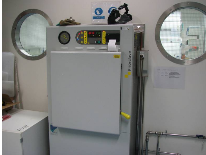
Figure 3: Double-ended autoclaves are fitted in Containment Level 3 and 4 laboratories
