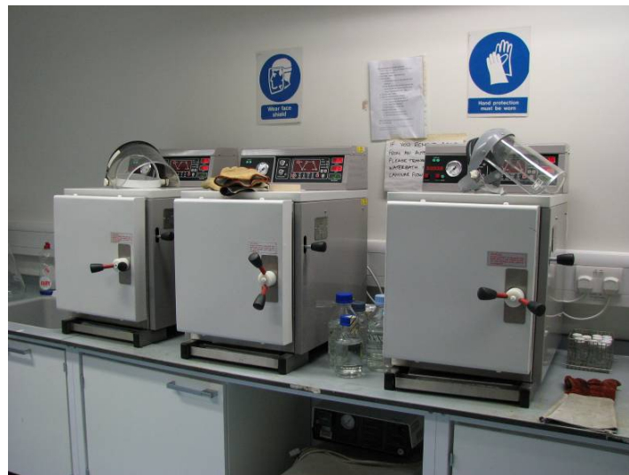
Figure 1: Bench top autoclaves used for media preparation and sterilization of instruments and pipette tips.
