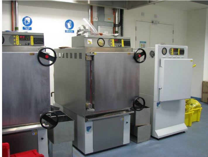
Figure 2: Autoclaves used for the inactivation of infectious and genetically modified agents.
